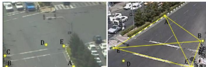
Figure3. Five Control Points in overlapping fields of view
