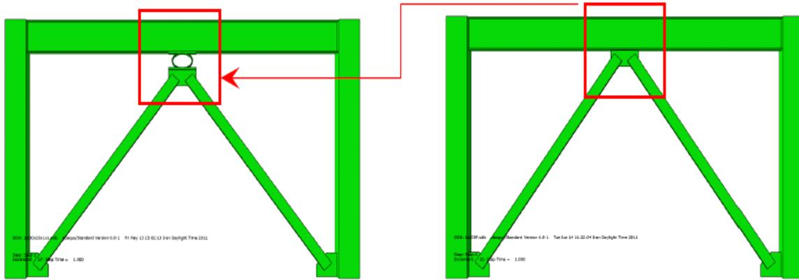
Figure 1. Placement of the damper in the braced frame
