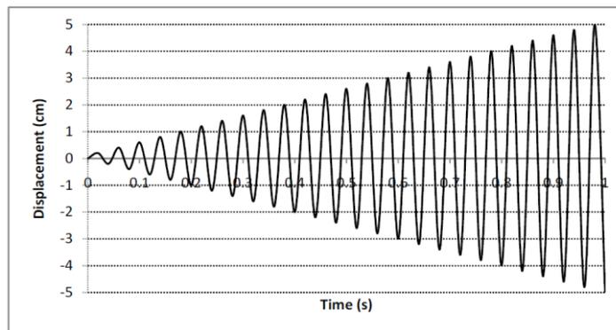
Figure 5. Applied loading diagram
