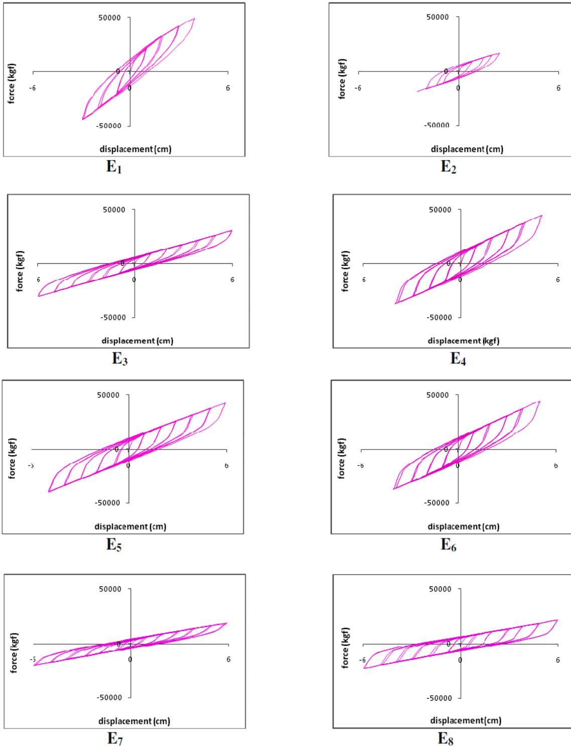
Figure6. Hysteresis loop of loading-displacement of the frame
