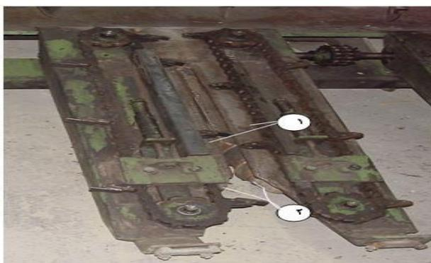
Figure 3. System for separating the cobs from the stalk
