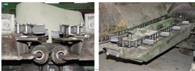
Figure 10. Chain tightener spring mechanism
