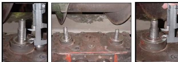
Figure 12. Mounting the gearbox when the axes' altitudes vary
