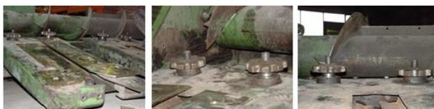
Figure 14. Mounting the roller chain when the altitudes vary
