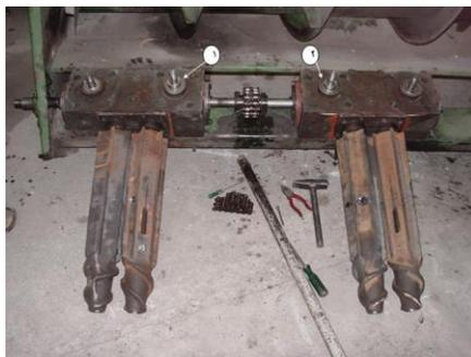
Figure 13. Mounting the sprockets and the gearbox
