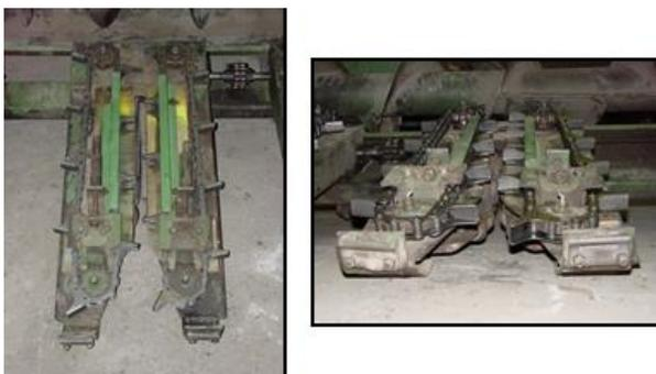
Figure 15. Mounting all feeder unit plates
