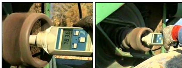
Figure 18. Reading the threshing drum's rotation and optimizing it for harvest
