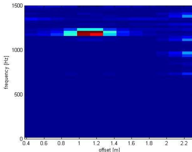
Figure 2: Power spectral density function of a buried cavity.
