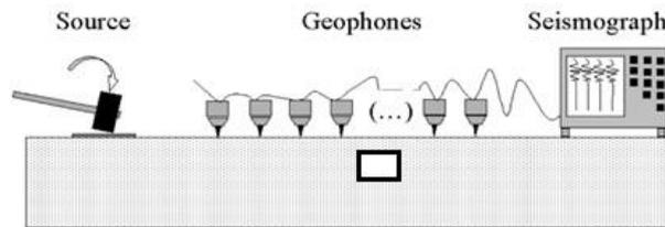
Figure 1: schematic image of the MASW test setup
