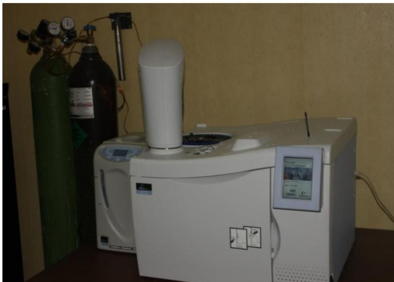
Figure 4. The Gas Chromatograph used for oil and produced biodiesel analysis.
